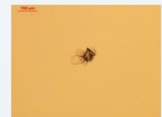
Optical microscopy images of impacted surface of RLA1 and RLB1 samples exposed according to north direction in Ouarzazate site
