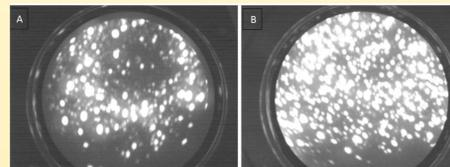
Fig. 12. FIM pattern structure for composite emitter 4 (Tungsten/ 478 Resin), the thickness of epoxy layer is 30 nm. Primarily consists of a multi big and bright spot. A) Applied field is 4000 V and temperature is 75K. B) Applied field is 5000 V and temperature is 75K
