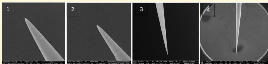
Fig.1: SEM images for uncoated emitters from 1 to 4.
