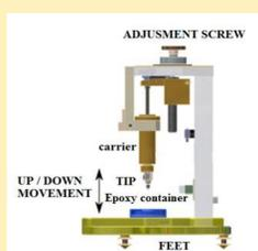
Fig.4 The setup used for coated the W tips.
