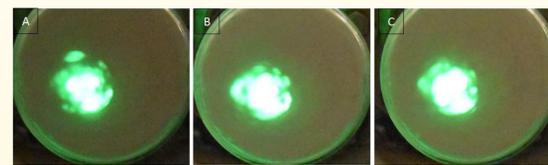
Fig. 9. FEM pattern structure for uncoated emitter 2 primarily consists of a multi spots. A) 2.2  $\mu$ A at 2,200 V. B) 2.4  $\mu$ A at 2,400 V. c) 2.9  $\mu$ A at 2,500 V. Time separation between consecutive images is 15 minutes.
