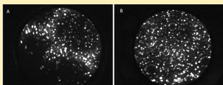
Fig. 7. FIM patterns for uncoated emitter 2 primarily consists of a multi small spots, A) Applied field is 3.5 kv and temperature is 75 k B) Applied field is 5 kV Applied field is 75k.
