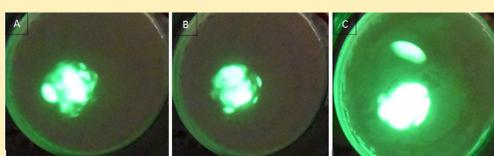
Fig. 5. FEM pattern structure for uncoated emitter 1 primarily consists of a multi spots. A) 2  $\mu$ A at 2,000 V. B) 2.3  $\mu$ A at 2,200 V. c) 2.7  $\mu$ A at 2,500 V. Time separation between consecutive images is 15 minutes.
