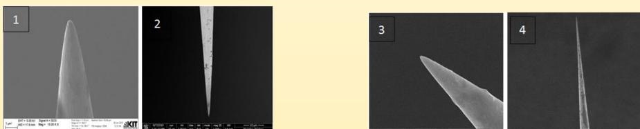
Fig.2: SEM images for composite emitters 3 and 4 (tungsten / UPR-4 resins), the thickness of epoxy layer is 150 and 30 nm respectively.
