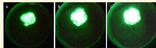
Fig. 10. FEM pattern structure for composite emitter 2 (Tungsten/ 478 Resin), The thickness of epoxy layer is 150 nm. Primarily consists of a single bright spot. A) 4.3  $\mu$ A at 2,300 V. B) 5.4  $\mu$ A at 2,500 V. c) 6.8  $\mu$ A at 2,600 V. Time separation between consecutive images is 15 minutes.
