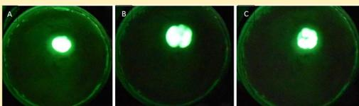
Fig. 6. FEM pattern structure for composite emitter 1 (Tungsten/ UPR- 4 Resin), the thickness of epoxy layer r is 150 nm. Primarily consists of a single bright spot. A) 3.2  $\mu$ A at 2,000 V. B) 4.4  $\mu$ A at 2,400 V. c) 5.6  $\mu$ A at 2,500 V. Time separation between consecutive images is 15 minutes.
