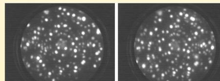
Fig. 11. FIM patterns for uncoated emitter 4 primarily consists of a multi small spots, A) Applied field is 3.2 kv and temperature is 75 k B) Applied field is 5.3 kV and temperature 75k.
