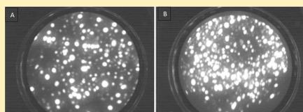
Fig. 8. FIM pattern structure for composite emitter 4 (Tungsten/ 478 Resin), the thickness of epoxy layer is 30 nm. Primarily consists of a multi big and bright spot. A) Applied field is 4000 V and temperature is 75K. B) Applied field is 5000 V and temperature is 75K.
