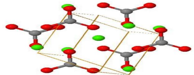
Fig.1 Rhombohedral unit cell of calcite (m space group), containing six units and seven Ca++ ions
