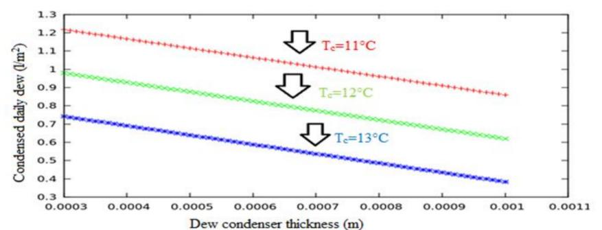
Fig 1 : The net effect of condenser thickness on estimated dew yield at three different values of condenser temperature T<sub>c</sub>.
