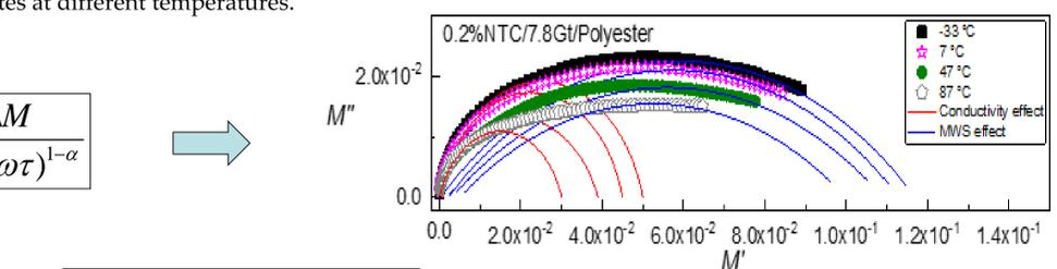
Fig. 4. Nyquist plot of the complex electric modulus of 0.2%CNT/7.8%Gt/Polyester composite. Solid lines are fits to the Cole-Cole model.
