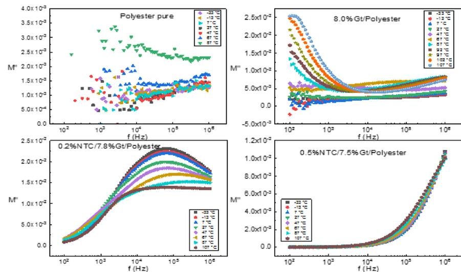
Fig. 3: Imaginary part of the electric modulus,  $M''$ , as a function of frequency for pure Polyester, GT/Polyester and CNT/Gt/Polyester composites at different temperatures.
