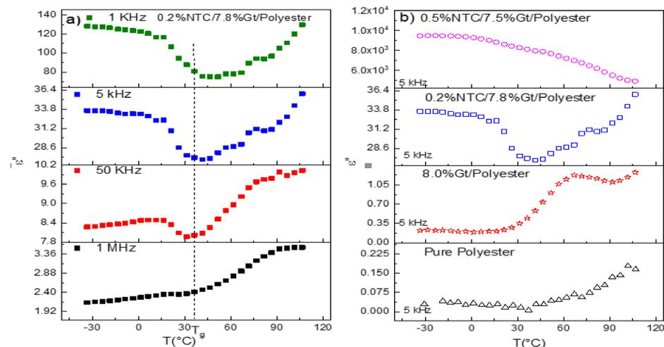
Fig. 2: Temperature dependence of imaginary part of dielectric permittivity: (a) for 0.2%CNT/7.8Gt/Polyester at different values of frequency, (b) comparative curves of each sample at 5 kHz.
