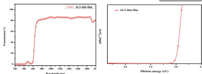
**Figure 1:** transmission spectra and band gap of ALS film deposited by spin-coating on a glass substrate
