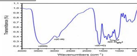
**Figure 4:** FTIR spectra of ALS powder
