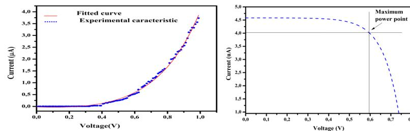
**Figure 5:** comparison of I-V characteristics of the solar cell in darkness and lighting
