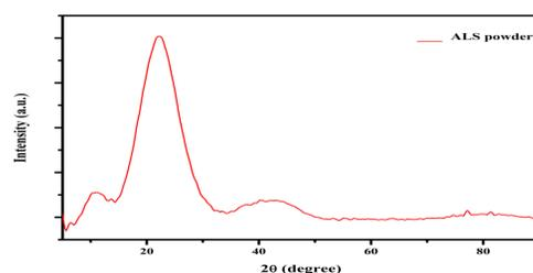
**Figure 3:** the X-ray diffraction spectrum of ALS powder
