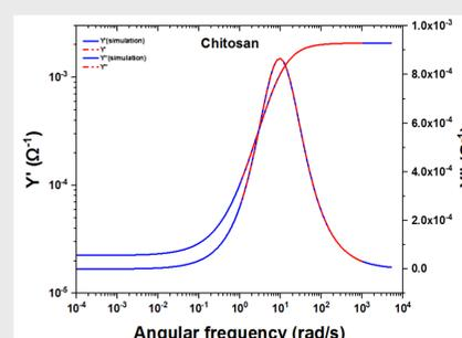
Figure 2. reel and imaginary part of impedance and admittance as a function of angular frequency of Chitosan and Gum Arabic
